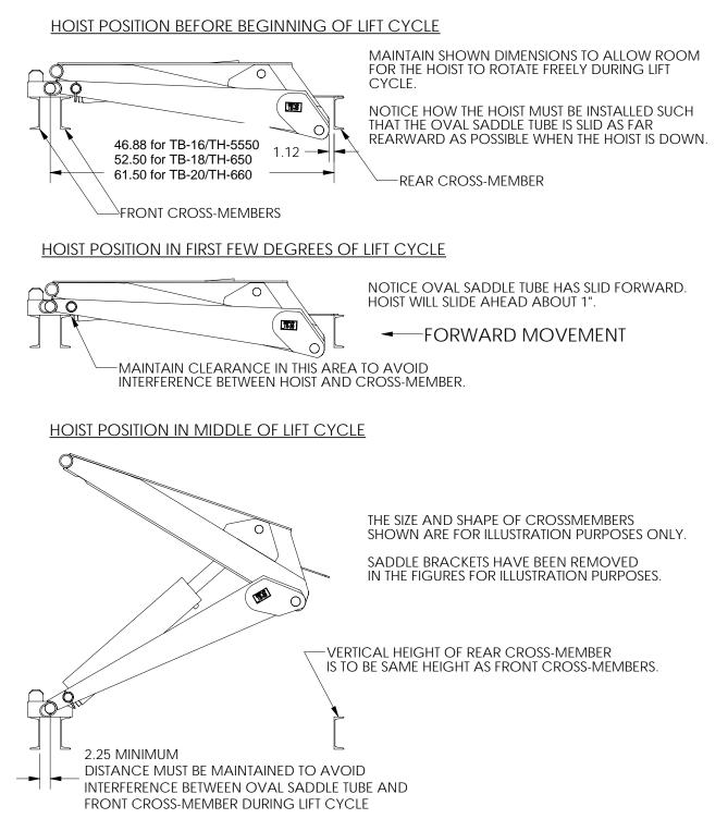
**NOTE:** The cross-members mentioned above are not supplied with the hoist, as they are part of the trailer design. For a given trailer, these cross-members must be of sufficient strength to support the hoist and any possible load that the cross-members will have on them during the dumping of the trailer.
