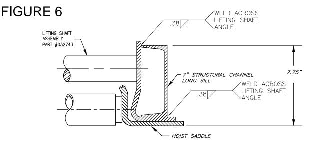
HOIST TO BODY ATTACHMENT DETAIL FOR 7" STRUCTURAL CHANNEL LONG SILLS AND 7.75" MOUNTING HEIGHT.
