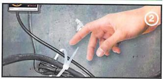
If needed, use plastic cable ties (not included) to secure the circuit box wires to the battery cable or other secure area near the battery. This will keep the wires from being damaged or interfering with any moving engine parts.
