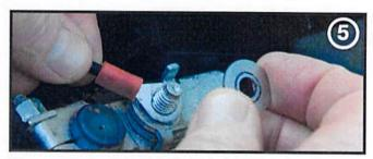
Slip a round washer (not included) onto the bolt until it sits next to the lug. Replace the nut onto the bolt and tighten it until it secures the lug and washer against the clamp. Do not over tighten. Repeat steps 4-5 above to connect the negative (-) black SolarPulse wire to the negative (-) battery terminal.
