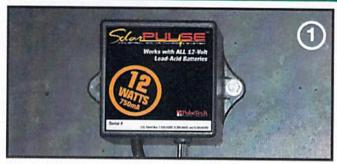
The circuit box can be mounted using any of the following methods: Two round-head screws, industrial adhesive, heavy-duty dual lock or double-sided tape (not included). After cleaning the install area, mount the box close to the battery so that the lugs can reach the terminals. DO NOT attach it to the battery itself. Also make sure the box is located in a location where it won't be disturbed and the LED is visible.
